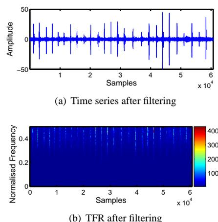
Fig. 5. Filtered footstep data from walking in boots on concrete at 2 feet from sensor
