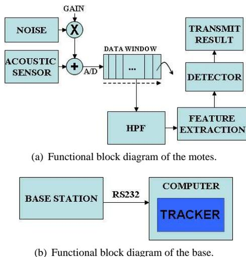
Fig. 3. Schematic block diagram of functional units.
