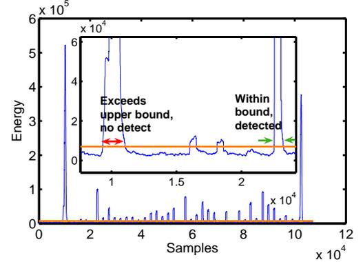
Fig. 6. Energy levels of footstep data at each time window
